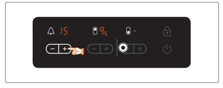
To display the time remaining for any of the cooking zones, use the timer's control sensor  $\triangle$ . The corresponding control indicator will begin to blink slowly.
